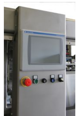
Repeatable and Easy Changeover via Standard 10" Color Touch Screen HMI
